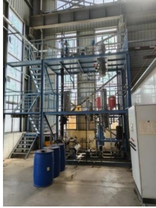
Fig.1. Ammonia-water absorption refrigeration experimental platform
