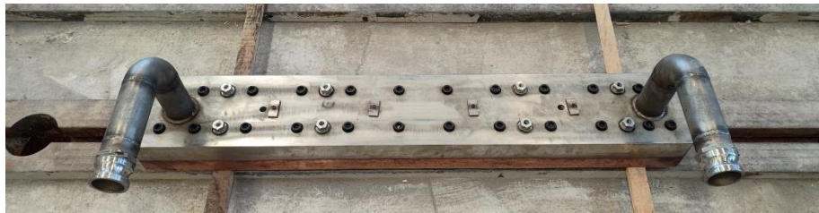
Figure 4. Photograph of the physical prototype of the water-channel crystallizer copper plate
