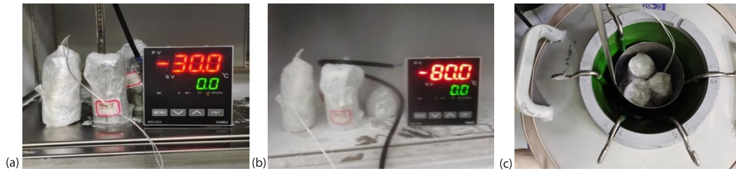
Figure 4. Gradient refrigeration of the specimens; (a) primary refrigeration, (b) secondary refrigeration, and (c) tertiary refrigeration
