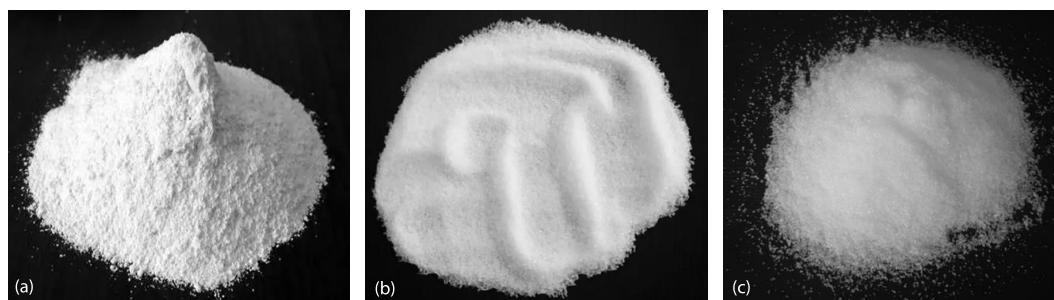
Figure 2. Inert dust samples; (a) CaCO 3 , (b) NaCl, and (c) NH 4 H 2 PO 4
