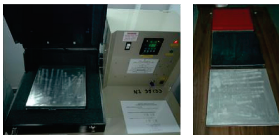
Figure 17. The Hilton B480 unit and samples 300 \times 300 \times 26 mm
