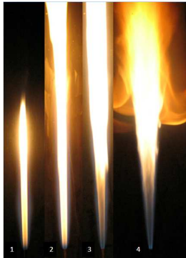
Figure 10. Variations of propane flame configuration with jet injection velocity U_j . Oxidant stream composition is 60 molar percent of oxygen and 40 molar percent of nitrogen. Oxidant stream velocity is 6 cm/sec. 1) Re_j = 1879 , 2) Re_j = 2369 , 3) Re_j = 7066 , 4) Re_j = 16500
