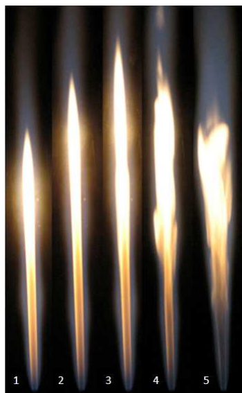
Figure 4. Variations of natural gas flame configuration with jet injection velocity U_j . Oxidant stream composition is 60 molar percent of oxygen and 40 molar percent of nitrogen. Oxidant stream velocity is 6 cm/sec. 1) Re_j = 1403 , 2) Re_j = 1683 , 3) Re_j = 1830 , 4) Re_j = 2110 , 5) Re_j = 2818
