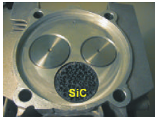
Figure 13. View of engine head with SiC ceramic material mounted in space between valves (Courtesy: F. Durst, [5])
