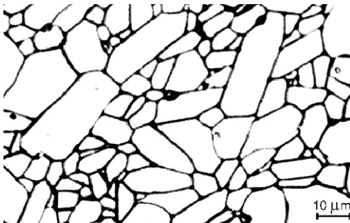
Figure 7. Microstructure of aluminium oxide ceramic (99.7%) (Courtesy: Brevier Technische Keramik)
