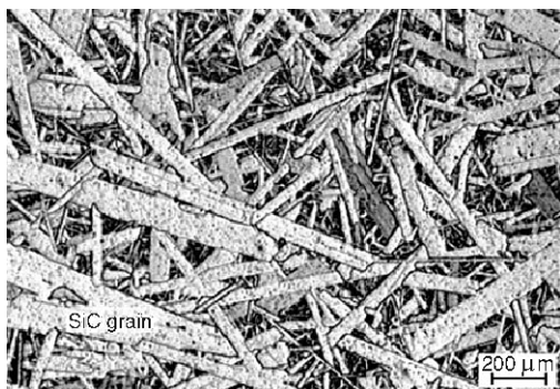
Figure 8. Microstructure of coarse-grained SSiC (etched) (Courtesy: Brevier Technische Keramik [20])
